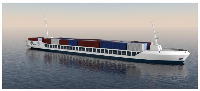
Length Overall 90.0 metres Draft mid. 5.50 metres Service Speed 10.5 knots (85% MCR)
