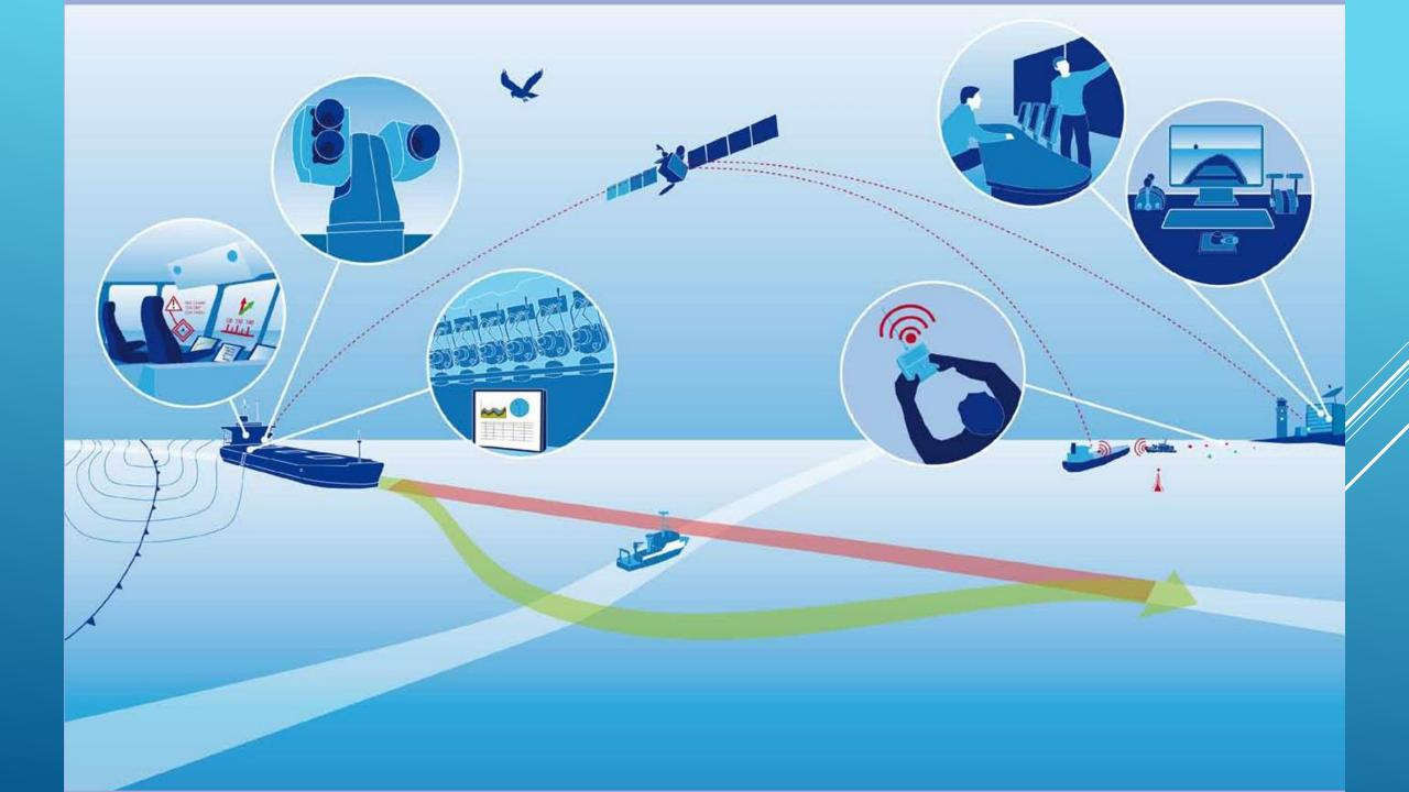
• An Advanced Sensor Module, which takes care of the lookout duties on board the vessel by continuously fusing sensor data from existing navigational systems, such as radar and AIS, combined with daylight and infrared camera imagery;
